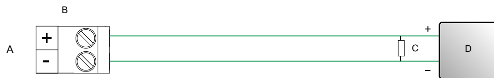
Figure 3-4: Internally-powered FO wiring
