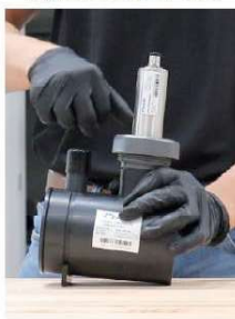
Tighten Sensor Nut
