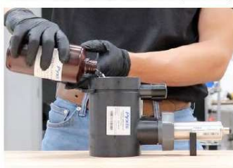
Add Calibration Standard (500mL)
