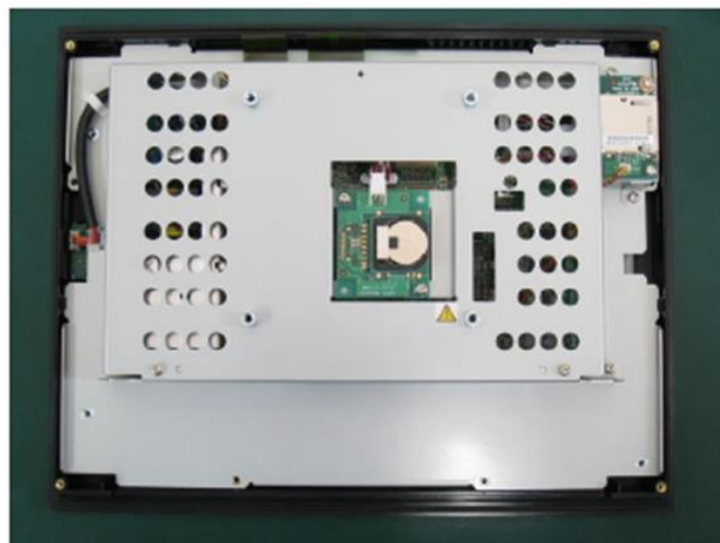
Figure 72: Coin Battery Location IC755CxSxxCDx
