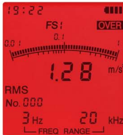
Overload indication screen
