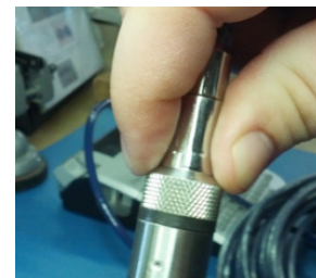
Properly completed—black ring uncompressed
